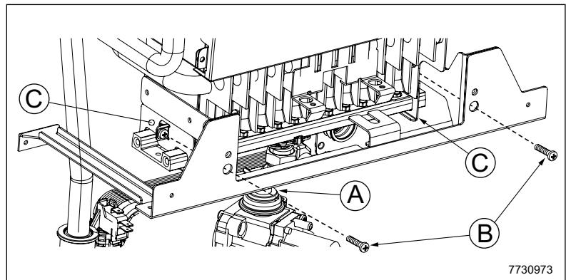
**WARNING:** do not unscrew the nozzles from the nozzle unit. The whole nozzle unit must be replaced.
