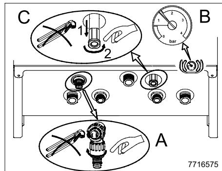
**Take special care when filling the heating system. In particular, open any thermostat valves in the system, ensure the water enters slowly in order to prevent the formation of air inside the primary circuit until operating pressure is reached. Lastly, vent any radiators in the system. Our company declines all liability for damage deriving from the presence of air bubbles in the primary exchanger due to the incorrect or imprecise observance of the above.**
